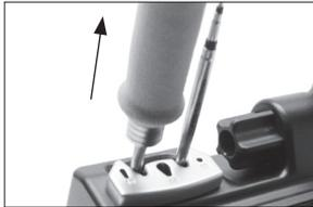
Place the handpiece in the extractor and pull to remove the cartridge.
