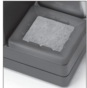
The least harmful cleaning method. Keep the sponge damp with distilled water when working to avoid tip wear.
