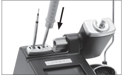
Place the handpiece on top of the new cartridge, press it slightly down and remove the handpiece from the extractor.
