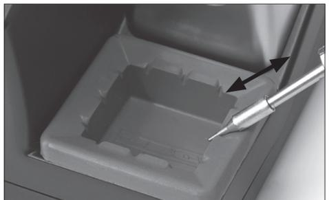
Use the slots to wipe any possible particle stuck on the tip.
