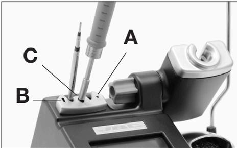
Press the cartridge into the opening A, B or C:
