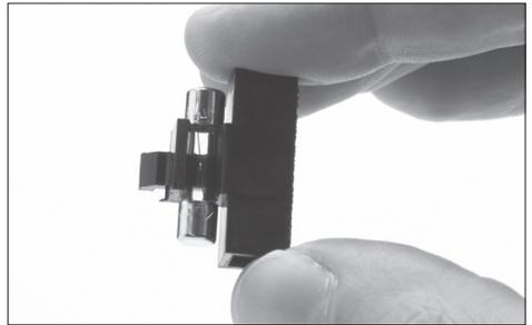
Place the new fuse into the holder by pushing and place it again into the station.
