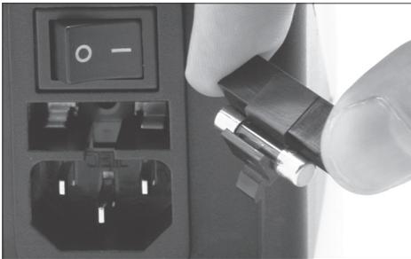
Unplug the station. Remove the fuse by pulling the black cap. Help yourself with a lever tool if necessary. See the fuse's technical specifications on the last page.
