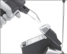
When the tool is lifted from the stand the tip will heat up to the selected temperature.
