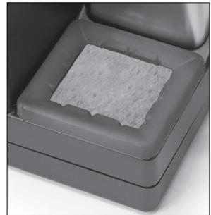
The least harmful cleaning method. Keep the sponge damp with distilled water to avoid tip wear.
