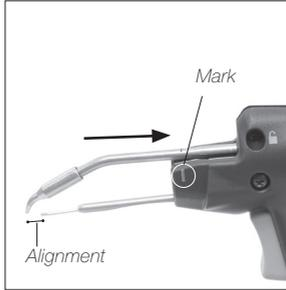
**Important:** Insert the cartridge as far as the mark for a correct connection.
