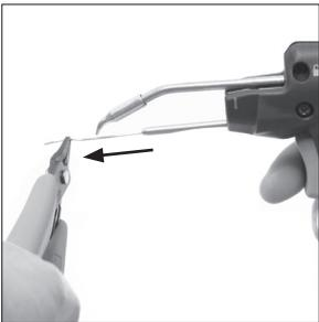
Pull out the remaining solder wire from the feed tube. Use a pliers if necessary.
