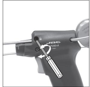
**Important:** Tighten the screw again being careful not to over-tighten. This is necessary for the tool to function.
