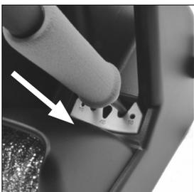
Place the handpiece on top of the new cartridge and press down slightly.
