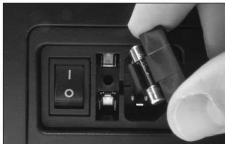
**2.** Press the new fuse into the fuse holder and replace it in the station.
