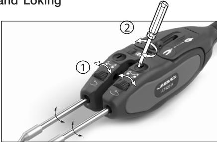
① Slightly turn the wheels to align the cartridges as required. ② Lock the fixing screws\*.
