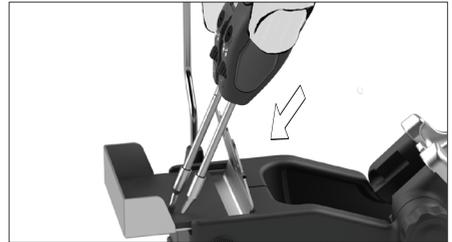
Lift up the Tweezer and press against the stand to insert the cartridge until you reach the mark\*.
