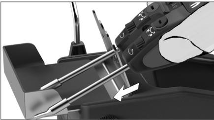
Use the grooves to position the cartridges.
