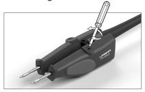
Unlock the fixing screws.
