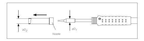
If the outer cartridge diameter  $D_1$  is larger than the inner nozzle diameter  $D_2$ . The cartridges must be removed first before the nozzle can be removed.
