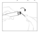
Introduce a small shaft or screwdriver, not deeper than 8 mm, and lift and pull out the sealing plug. Never use a cartridge to do this operation.
