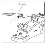
Loosen the handle screw. Place the soldering iron with the cartridge in the extractor and pull the handle to remove it.
