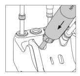
Place the handpiece on top of the new cartridge and press down slightly.
