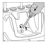
Use the holes to fix the cartridge at the right depth (1). The extractor holes also allows correcting the nozzle angle of curved cartridges. To do this, rotate the tool (2) with the cartridge inserted in the extractor until the nozzle is in the right position.
