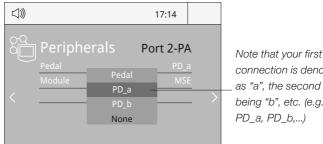
connection is denoted as "a", the second being "b", etc. (e.g. PD a, PD b,...)
