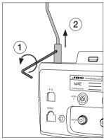
Loosen the set screw (1) and withdraw the cable collector (2).
