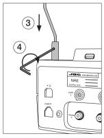
Insert the new cable collector (3) and tighten the screw (4).
