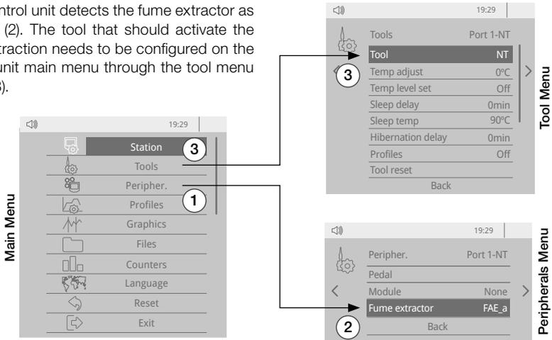
Connect up to 4 control units (connector FAE/ROBOT) to the fume extractor connectors (STATION 1, STATION 2, ...). Each tool connected to these control units can start and stop the fume extractor.
