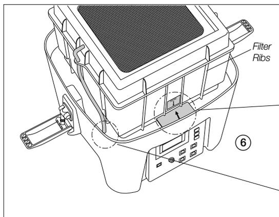
**Note:** The main filter has a given position. Make sure the filter ribs mate with the corresponding slots of the casing.
