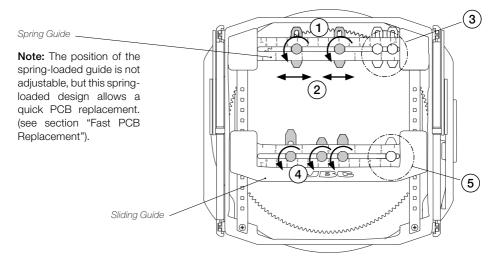
Insert the PCB into the slots of the spring guide clamps (6) and into at least one clamp on the side of the sliding guide (7) and tighten the clamp knob (8).
