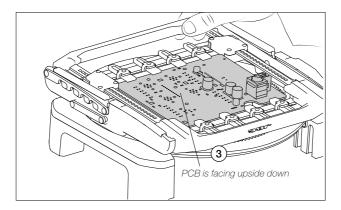
**Note:** Pay special attention when turning the PCB so that components do not collide with the working surface or with PHSE Preheater (if used). If necessary, set a different support height or angle.
