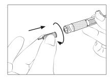
1. Replace the cap of the barrel (or the needle/tip in use) with the new needle/tip.
