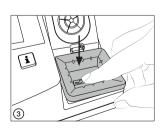
At the station's bottom side, pull on the tab to attach the wiper and secure it in place (4).
