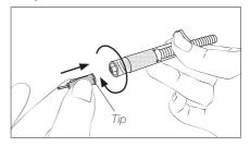
Screw the tip onto the syringe barrel.
