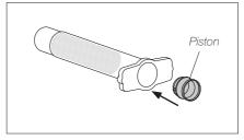
Fit the piston into the barrel.
