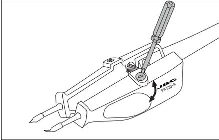
Unlock the fixing screws.
