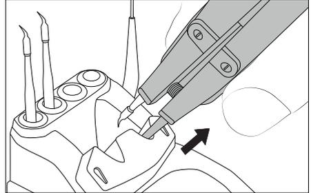
Place the cartridges in the extractor and pull the tweezers to remove the cartridge.
