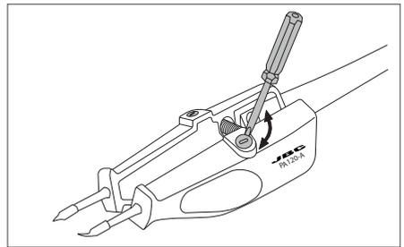
Lock the fixing screws.
