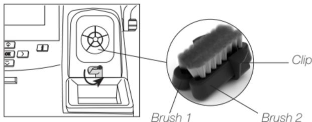
\* **Note:** To join 2 brushes the connection clip is needed. Ref. CL6217 does not include any clip. Reuse the clip of your worn brushes.
