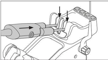
Once the previous cartridges are removed from the stand, insert the new cartridges into the two outer grooves. Position the tweezers over the cartridges and press it onto them.
