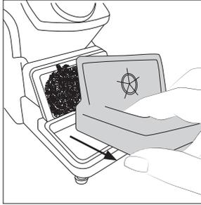
Remove the wiper by pulling it out.
