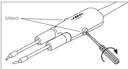
Finally lock both cartridge fixing screws.
