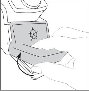
Lift the wiper at its front edge.
