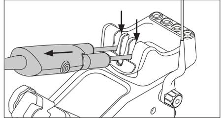
Place the cartridges in the two outer grooves and pull the tweezers to remove the cartridges from the tool.
