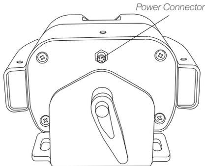
The connector provides “switch” input and power supply.
