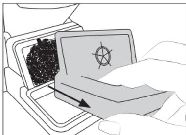
Remove the wiper by pulling it out.
