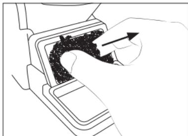
Replace the brass wool with a new one when it is worn out.
