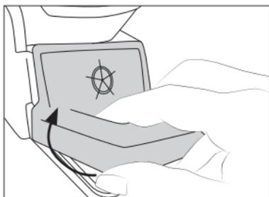
Lift the wiper at its front edge.
