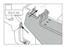
Separate both parts of the cleaning system to remove the brush.
