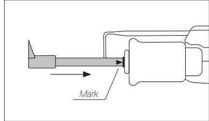
Insert the cartridge until the reference mark. Take the mark as reference and check that both tips match.
