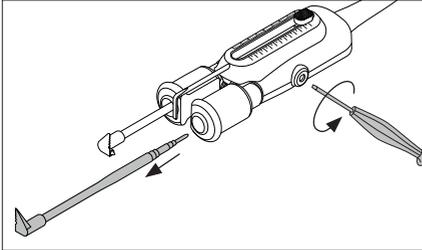
Loosen the screws and remove the cartridges.
