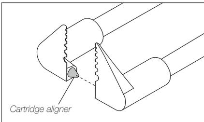
Align the cartridges in working position using a flat pliers (JBC Pliers PLR195). The conical cartridge aligner helps centering both cartridges and ensure a good functionality.
