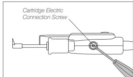
Fix the cartridges in its working position by tightening the screw.
