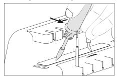
Tilt the handle slightly towards you until the cartridge releases from the clamp.
