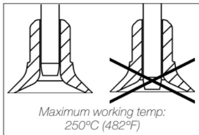
For a correct suction process insert the needle in the cup as shown in the picture.
