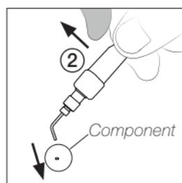
Once the suction is activated, cover the pen hole with your finger (1) and lift off the component.
