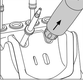
Place the cartridge in the extractor and pull the handle to remove it. Use the ring (J325) or umbrella (J125) around the cartridge as a stop to extract it from the tool.
