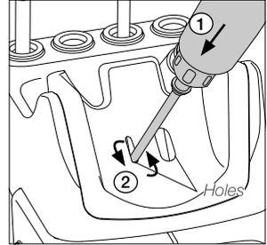
Use the holes to fix the cartridge at the right depth (1). The extractor holes also allows correcting the nozzle angle of curved cartridges. To do this, rotate the tool (2) with the cartridge inserted in the extractor until the nozzle is in the right position.
