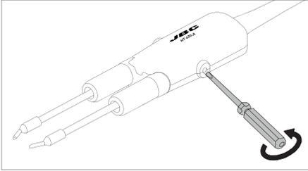
Unlock the fixing screws.
