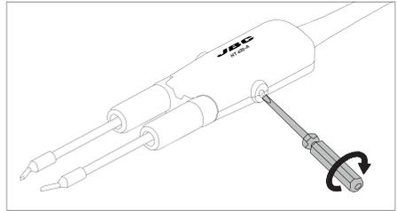
Lock the fixing screws.
