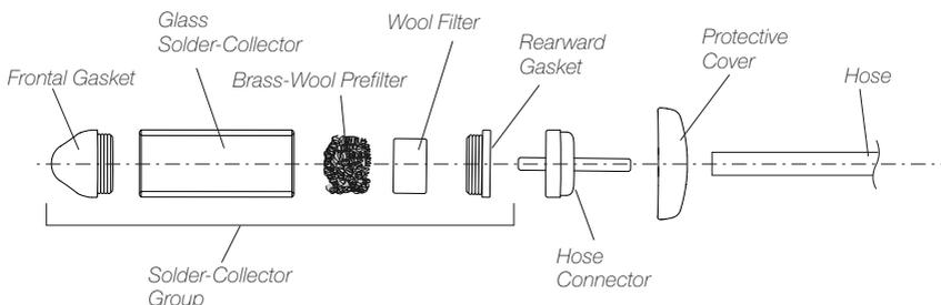
**Note:** To position the brass-wool prefilter correctly, remove the front gasket push it against the wool filter. Reassemble the front gasket.
