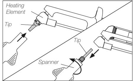
If the heating element has a tip on, remove it with the provided spanner.
