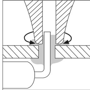
As the solder joint liquefies, gently describe circles around the pin, using the pin as the axis of your movement.
