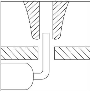
After releasing the tool button there is a slight delay until the vacuum pump of the desoldering module stops. This makes sure that the tip duct is completely empty.
