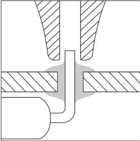
Place the tool so that the end of the component's pin fits inside the desoldering tip.
