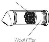
**\*Note:** Brass-wool and metal-sheet prefilters can be cleaned by shaking off the loose solder residue. If they are too dirty, replace them with new ones.
