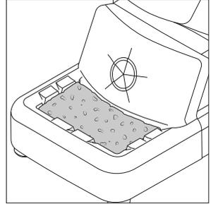
A damp sponge is the softest cleaning method. When working, keep the sponge damp using distilled water to avoid tip wear.
