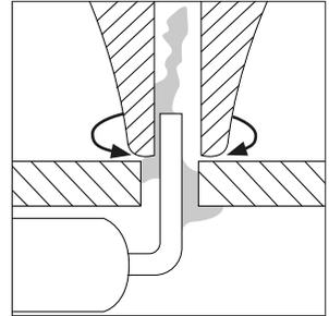
Press the tool button long enough to suction the liquefied solder.
