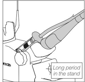
After longer periods of inactivity, the tool goes into Hibernation Mode: the power is cut off and the tool gradually cools down to room temperature.
