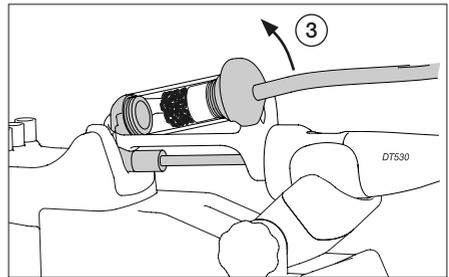
Then undock the frontal gasket (4) from the heating element to disassemble the solder-collector group.
