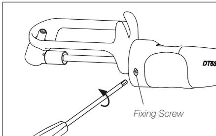
Loosen the fixing screw.
