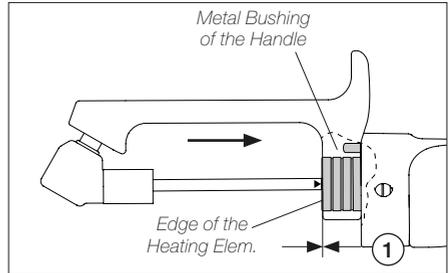
To fix the heating element in place, tighten the fixing screw.
