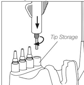
To remove the tip from the spanner, simply place the tip in one of the holes of the tip storage, screw it in lightly (only approx. 1 turn) and pull the spanner out.
