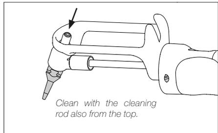
Remove the solder collector group, leave the tool on the stand and clean the tip with the cleaning rod also from its top.
