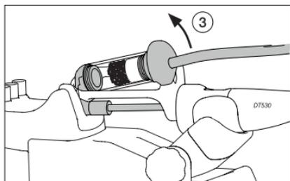
... and pull upward (3) to unlock the protective area.
