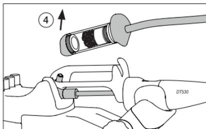
Then unlock the frontal gasket (4) from the heating element to disassemble the solder-collector group.
