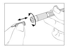
Replace the syringe cap for a stainless steel needle or a tapered tip.
