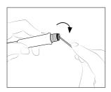
Enter a small shaft or screwdriver in order to gently lift and pull the Seal. Do not insert the tool more than 8 mm deep. Never use a cartridge to do this operation.
