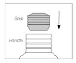
Note the Seal mounting position. The chamfered side has to be positioned towards the Handle.
