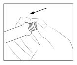
Gently push the Seal inside the handle until it is completely into the Handle. Handle and Seal edges have to be aligned.
