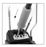
Place the handle on top of the new Cartridge and press down.
