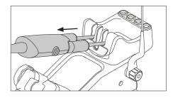
Place the cartridges in the quick tip changer and pull the tweezers to remove the cartridges.
