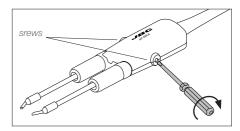
Lock the fixing screws.
