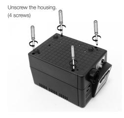
To have access to the connection you need loose the screws and release the frontal part carefully Carefully remove the housing.
