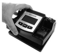
Place the housing without screwing. Plug the power cord. Plug the USB cord to the PC. Turn the station ON.
