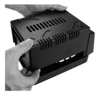
Place the lid without screwing. Plug the power cord. Plug the USB cord to the PC. Turn the station ON. Reprogram the station (see software manual).
