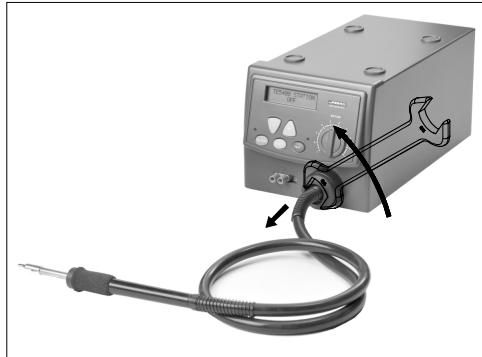
Move back the cover. Pull the connector from the socket to disconnect the heater from the station.
