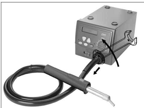
Move back the cover. Pull the connector from the socket to disconnect the heater from the station. Follow this process inverted to re-connect the heater.
