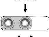
Two vacuum inlets available for tripods and extractors, being active the one that coincides with the arrow.
