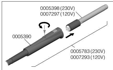
3. Connect the new heating element, pushing it's extreme.
