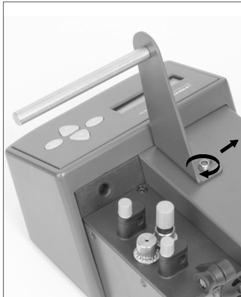
Place the toolholder metal base and the solder reel (maximum weight 1kg). Press the 2 screws.
