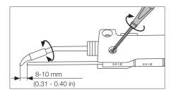
Align the cartridge tip with the solder guide tube. Leave a gap of 8-10 mm (0.31 - 0.40 in) between the tip and the end of the guide tube.
