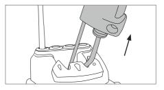
Place the cartridge in the extractor and pull the tool to remove the cartridge.
