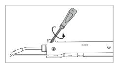
Unlock the cartridge fixing screw.
