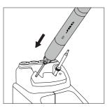
Use the holes to fix the heating element.
