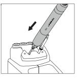
Place the handpiece on top of the new heating element and press down slightly.
