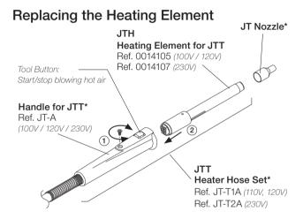
**Note:** Only perform this operation when the heating element is cold and the unit is disconnected from the mains.
