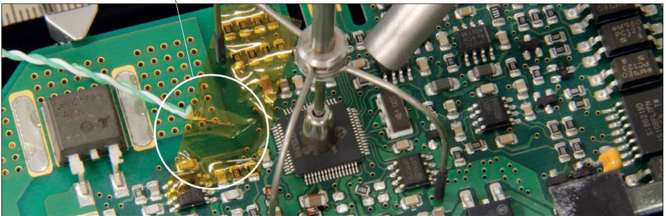
IPC\* does not recommend exceeding ramp-up rates over 3 - 4 °C / sec (5 - 7 °F / sec) so as to reduce the risk of thermal stress on the PCB.
