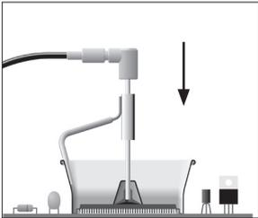
Position the extractor with the appropriate suction cup and press the suction button.
