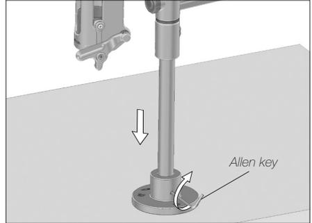
Fit the tool arm onto the flange and tighten the allen screw.
