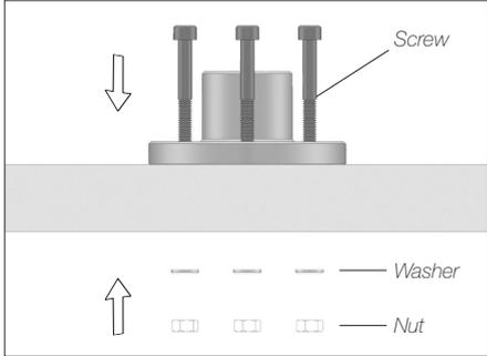
Fix the flange on your work table with the supplied screws, nuts and washers.
