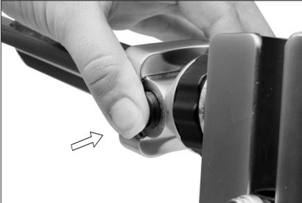
By holding down the button you can rotate the Tool Holder up or down.
