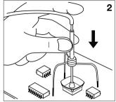
To desolder small components you must use the protector + tripod as shown in drawings 1 and 2.
