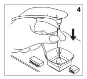
For bigger components use the extractors (fig. 3 and 4).
