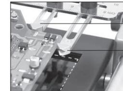
For fixing irregular shaped PCBs to the support.
