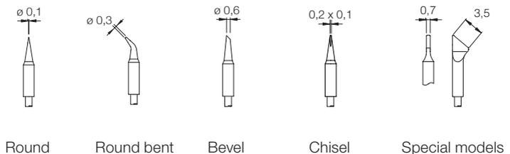
All the cartridges shown are actual size. All measurements are in millimeters (mm). Contact JBC if you need alternative shapes.
