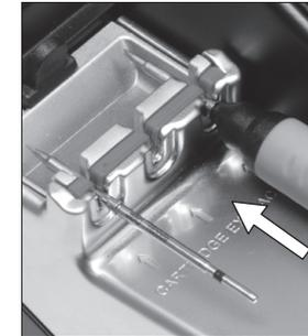
Push the cartridge into the slot and pull the handle to the mark\*.
