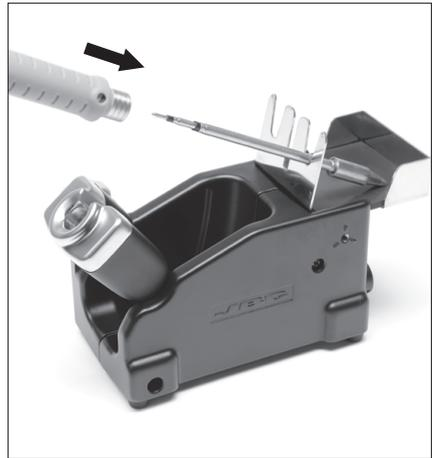
3 Place the handpiece on top of the new cartridge, press slightly down and remove the handpiece from the extractor.
