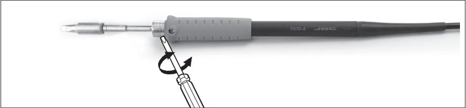
1 Untighten the screw before placing the handpiece in the cartridge extractor.
