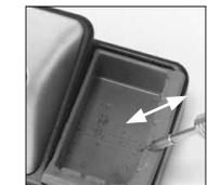
*Use the slots to remove remaining particles.*
