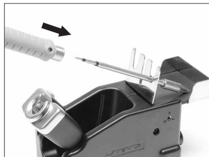
Insert the cartridge and press slightly until the mark\*
