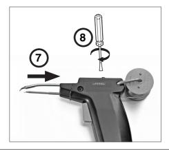
Please make sure that the soldering iron is not connected to the station. This step has to be performed when the cartridge is cold.
