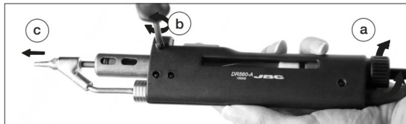
**Recommended:** Remove the lid in a vertical position and follow the cleaning guidelines in the tool and station manuals.
