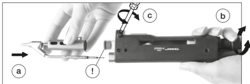
**!** **Important:** Before placing, make sure to insert the internal gasket into the Tin deposit.
