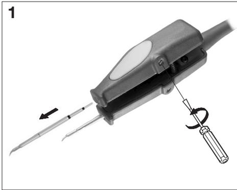
Loosen the cartridge screw to release the cartridge.
