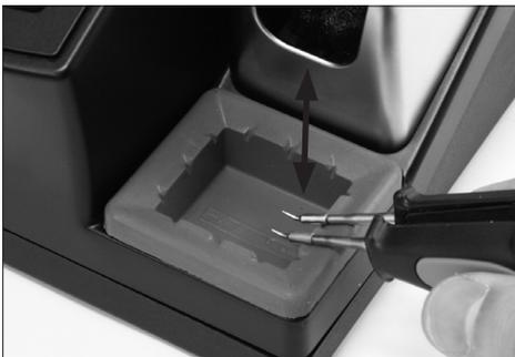
Tap smoothly the cartridge on the wiper profile to remove the excess of solder
