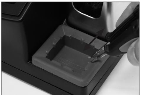
Use the slots to wipe any possible particle stuck on the tip
