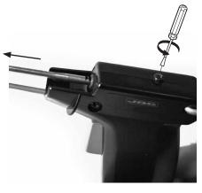
Loosen the screw and remove the cartridge.  $\triangle$  Use a flat pliers if still hot.
